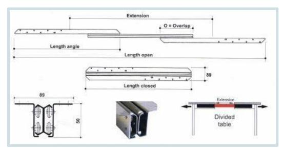
GQ-slides are developed for divided tables and are equipped with ball bearing steel rollers
