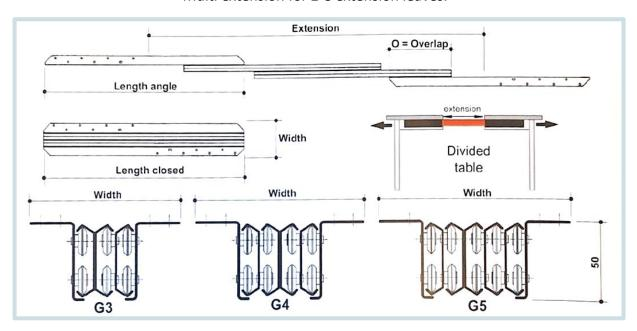
GQ-slides are developed for divided tables and are equipped with ball bearing steel rollers
